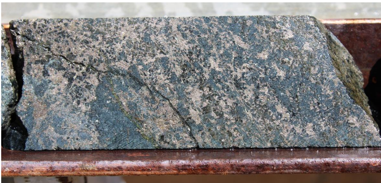
Figure 1: CNDD001A at 635.9m down-hole showing matrix-textured sulphide zone (NQ core ~48mm diameter)
