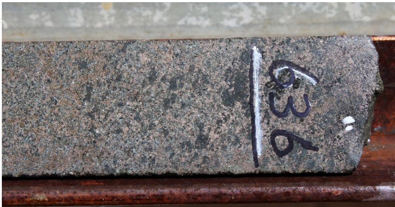
Figure 2: CNDD001A at 636.5m down-hole showing semi-massive sulphide zone
